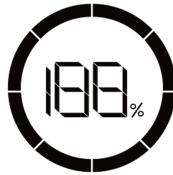
**Battery percentage:** This tells you what percentage of the battery's capacity is remaining. The circle around the battery will rotate when the battery is successfully charging.
